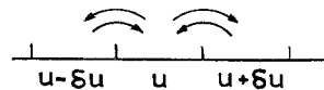
Figure 6 Possible transitions from and to a given energy level in the barrier-height distribution.
